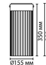
5047/10LC 1 x LED x 10W, 2715 lm крепеж: планка
