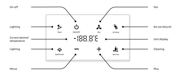
A typical configuration example for a sensor in a hotel application.
