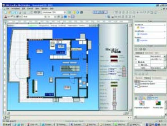
The visualisation editor presents the whole bus system as a model on the screen. The user has virtual access to devices and can make settings which apply to the bus system. The layout of the corresponding building can be shown for clear, convenient operation, and symbols for lighting, blinds or central heating can be allocated individually from an icon library.
