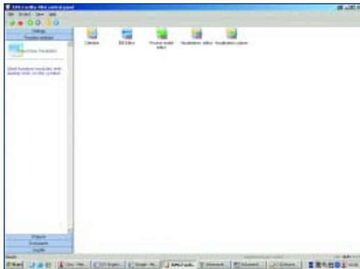
The JUNG Facility-Pilot is a flexible, interactive software for extensive visualisation and control of the building system technology KNX/EIB. Its areas of application extend from many different industrial applications through to up-market residential buildings. The software consists of individual modules such as the EIB editor, process model, visualisation editor and a comprehensive system control.
